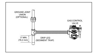
FIGURE 19. GAS PIPING WITH FLEXIBLE CONNECTOR.
